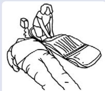
**Task 12.6.1a** Positioning the lifting cushion
